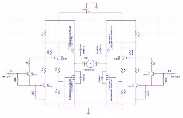
The H-bridge works by turning on a resistor voltage divider driving a voltage on each gate that exceeds the MOSFETs ON-gate voltage. The PWM input signal pulls the base of transistor T1 high which allows current to flow from the base of T3 to the base of T2, limited by a 5K $\Omega$  resistor. This turns T2 and T3 on, powering the voltage dividers comprised of R\_a/R\_b, and R\_c/R\_d.
