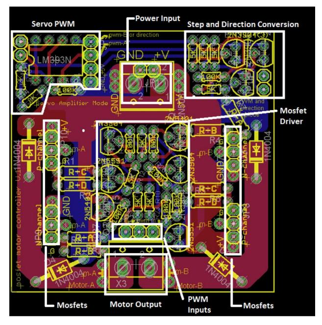
This is the Eagle CAD H-bridge schematic that we inherited from one of Dr. Luecke's previous students. We will use this as a starting point for creating a circuit design for our H-bridge. The Servo PWM and Step and Direction Conversion circuits in the drawing above do not work, so we will be omitting them from our circuit design.
